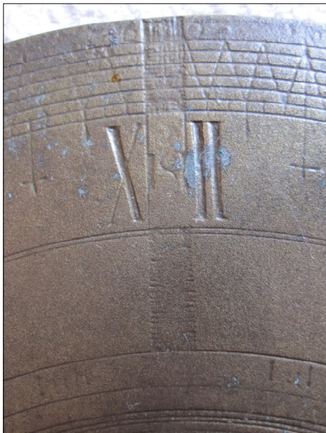
Fig. 14. Detail of the Ince Blundell dialplate showing the transversals and an "HS" monogram in the noon gap.
