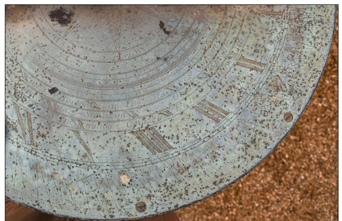
Fig. 7. A section of the Rowley 'geographic' dial at Blenheim Palace, dated 1710, with three rings marked with place names and their local noon times. The Silesian sundial strictly follows this pattern. Note the outward facing hour numerals and inward facing descriptions of the compass rose directions, again like the Silesian sundial.
