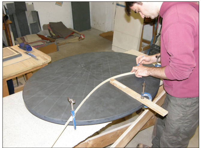
Fig. 6. Russell Purdham setting out the summer solstice curve.
