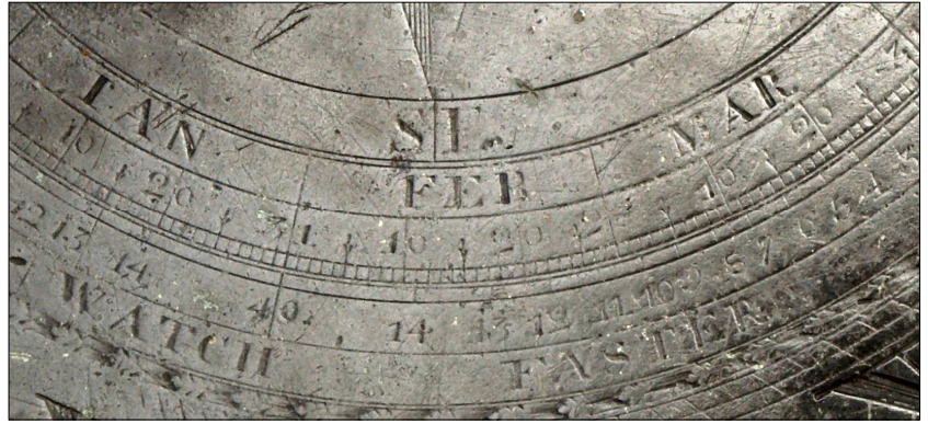
Fig. 5. Part of the EoT scale, showing the maximum of 14m 49s on 31 Jan.
